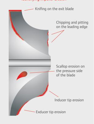
A timely inspection of critical components such as impellers can identify excessive wear and proper correction action to maintain efficient operation.
